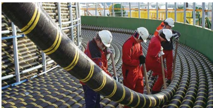
Figura 4 – Operários enrolando cabo umbilical (ABB, 2009).
